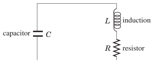
Fig. 1.2.7 A resonating circuit. A high Q value means that the circuit amplifies significantly only in a very narrow band around the resonant frequency \omega = 1/\sqrt{LC} .
