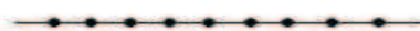
(c) Plane polarized light with electric field vibration perpendicular to plane of paper
