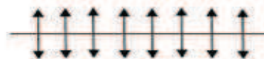
(b) Plane polarized light with electric field vibration parallel to plane of paper
