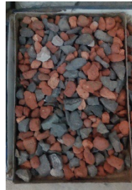
Figure-3: Appearance of Over-burnt bricks
