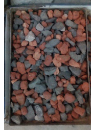
Figure-3: Appearance of Over-burnt bricks
