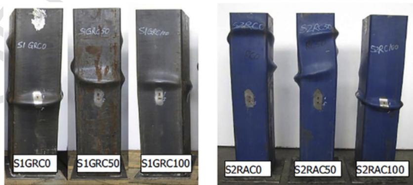
Fig. 5. Typical Failure Modes of Specimens under Axial Compression. X.S. Shi et al. (2015) [22].
