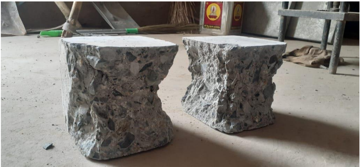
Fig . concrete cube after testing
