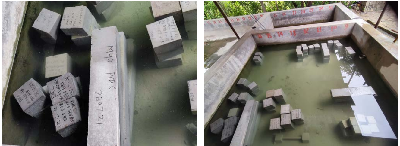
Fig. 9 PQC Sample Curing
