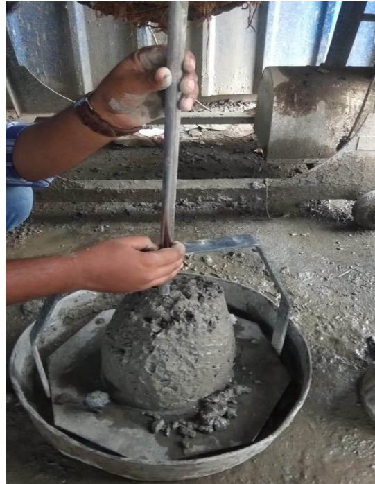
Fig . Testing of slump of concrete.
