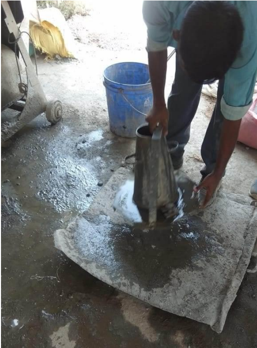
Fig . Testing of slump of concrete.
