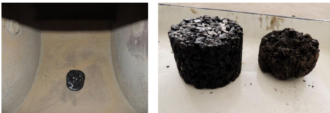
Figure 1 - (a) Specimen in abrasion cylinder (b) Fully compacted specimen and after abrasion.
