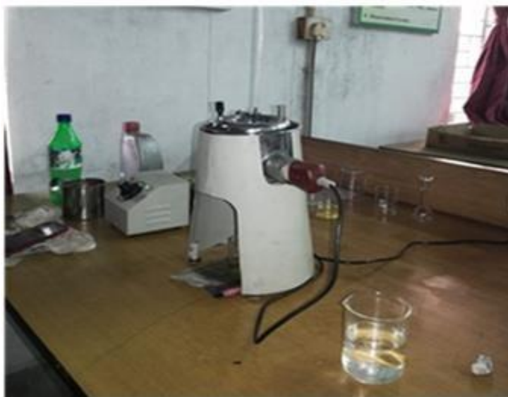
Fig.3: Experimental setup of Redwood Viscometer
