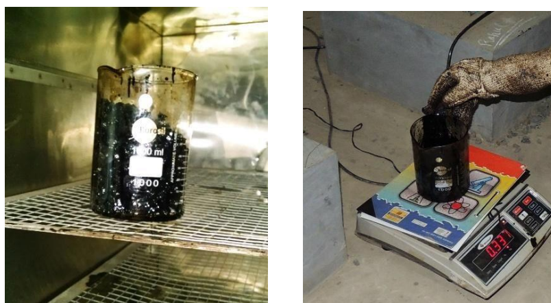
Figure 2 - (a) Specimen conditioning in oven (b) Flask with drained material.
