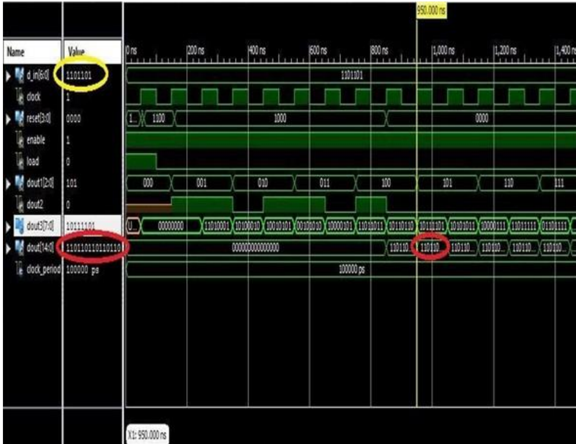
Figure-6 Simulation Result of BCH ENCODER
