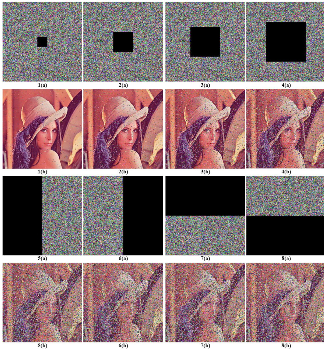
Fig. 10 Decrypted images “(b)” for occlusion size: 1(a) 32 \times 32 , 2(a) 64 \times 64 , 3(a) 96 \times 96 , 4(a) 128 \times 128 , 5(a) 50% left side, 6(a) 50% right side, 7(a) 50% top, and 8(a) 50% bottom
