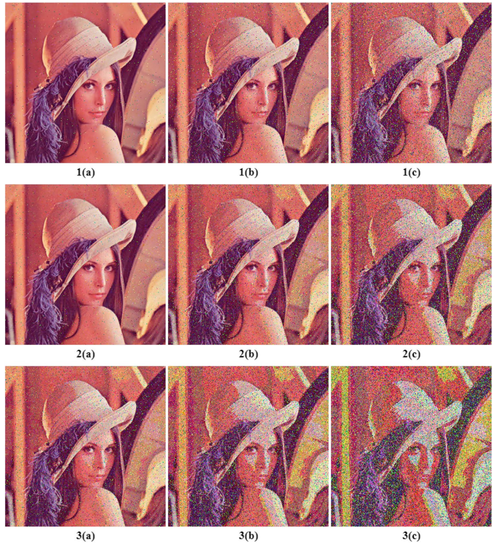
Fig. 9 Decrypted Lena images with different noises: Salt & Pepper noise with probability 1(a) 0.01, 1(b) 0.05, and 1(c) 0.15; Speckle noise with strength 2(a) 0.01, 2(b) 0.05, and 2(c) 0.15; Poison noise with lambda value 3(a) 5, 3(b) 15, and 3(c) 30
