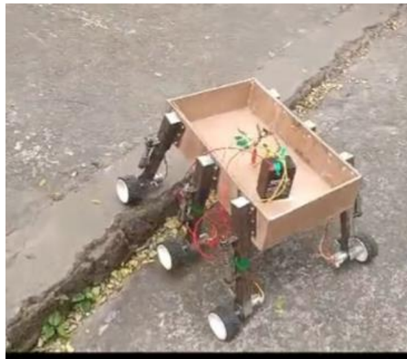
Fig. 2. Stair climbing nature of the rover
